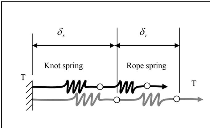
**Figure 23:** System of springs used to represent an anchor with knot slip.
