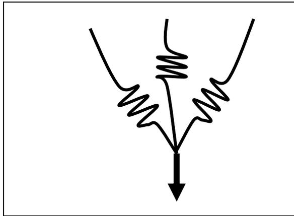
**Figure 21:** Anchor system viewed as a system of springs.
