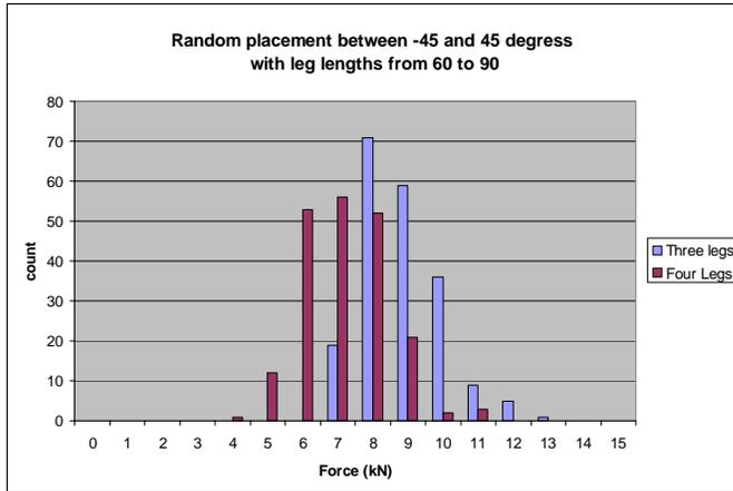
**Figure 28:** Maximum force in any given leg for a random placement in multi-point system.
