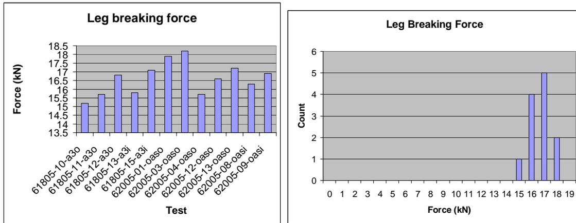
**Figure 20:** Failure force in a single leg of a three-point system pulled to failure; 20a (left) by individual test and, 20b (right) by total count.
