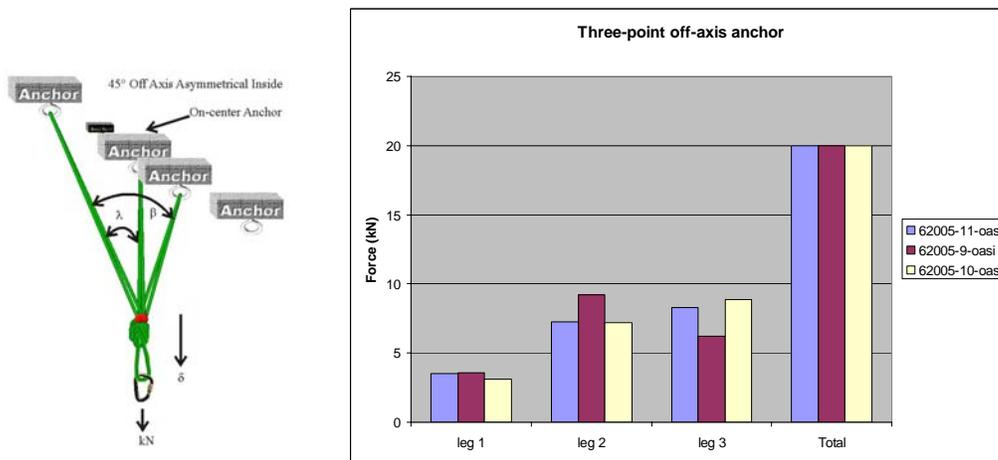
**Figure 12 and Figure 13:** Measured tensions in three tests of three-point off-axis asymmetrical inside ( $\beta/2 \neq \lambda$ ) anchor.
