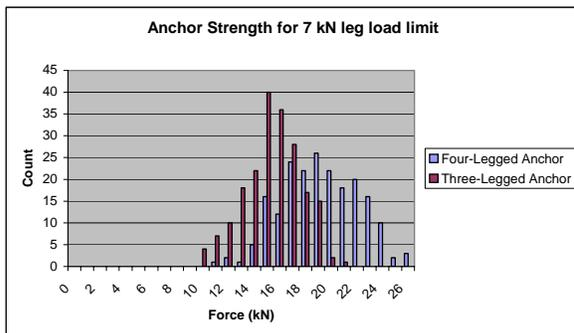
**Figure 29:** Anchor Strength with a limit of 7 kN in any given leg for 3 and 4 point anchors with random placement with angles between -45 and 45 degrees, leg length between 60 and 90 cm, and +/- 5 cm slack in each leg.
