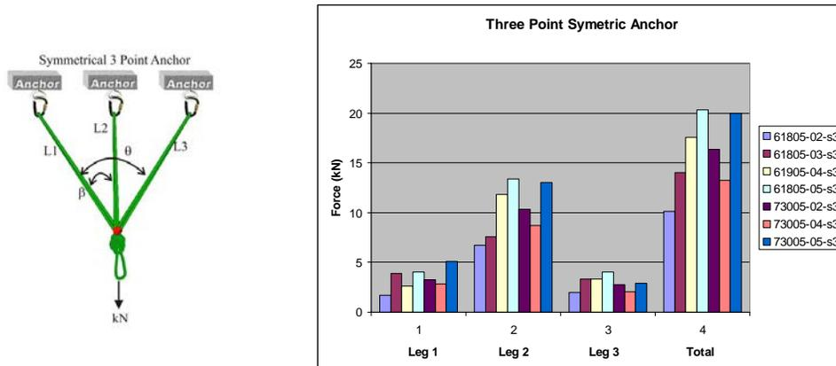
**Figure 3 and Figure 4:** Geometry and measured force from seven different symmetric three-point anchors system test.
