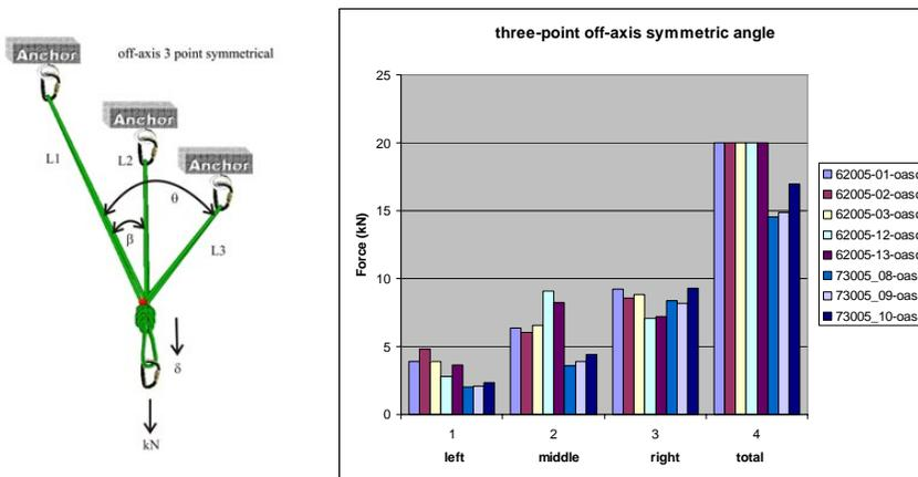
**Figure 8 and Figure 9:** Geometry and measured leg tension from eight different test of a three-point off-axis, symmetric angle ( $\beta=\theta/2$ ) anchor.
