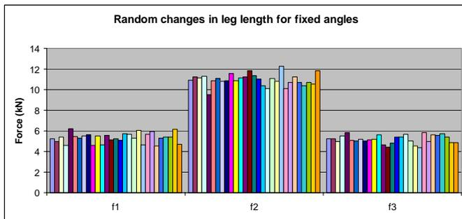
**Figure 26:** Effects on leg forces for a 3 point symmetric system from random changes in length of each leg by +/- 5 cm.
