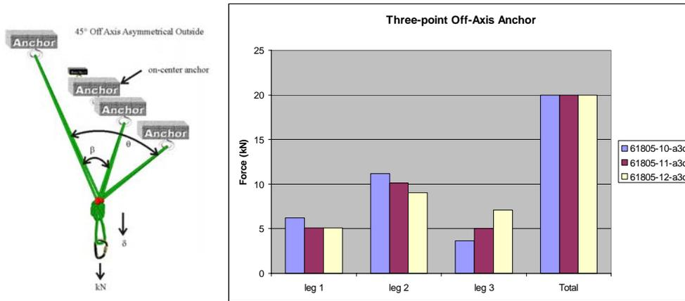
**Figure 10 and Figure 11:** Geometry and measured leg tension in three different test of three-point off-axis asymmetrical off-axis outside ( $\beta \neq \theta/2$ ) anchor.
