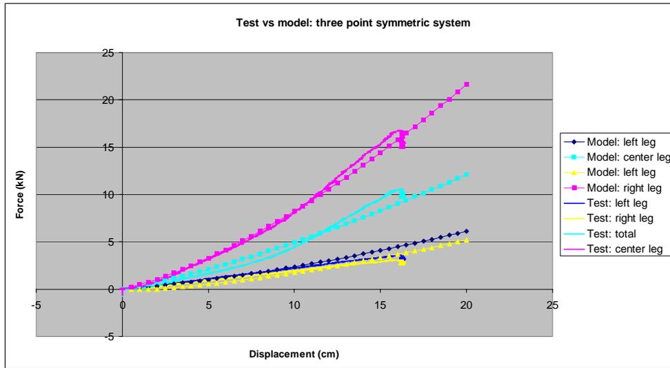
**Figure 24:** Example of knot slip and rope stretch computed using Equation 1.6 and 1.7. The model closely follows the test results.
