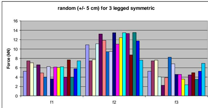
**Figure 27:** Effects on leg forces for a 3 point symmetric system from random changes in the initial slack in each leg (+/- 5 cm).
